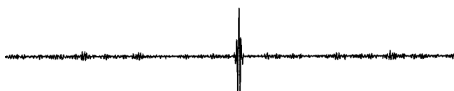
FIG. 7. Refocused signal obtained at A after a time-reversal of 1600 \mu\text{s} at B . The presented signal is about 210 \mu\text{s} long.
